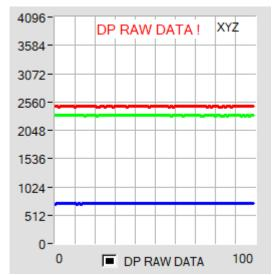
To understand with which **X**, **Y** and **Z** values the sensor works in parameter set 2, you can display this raw data in the tab **XYZ** using the **DP RAW DATA** check box.
